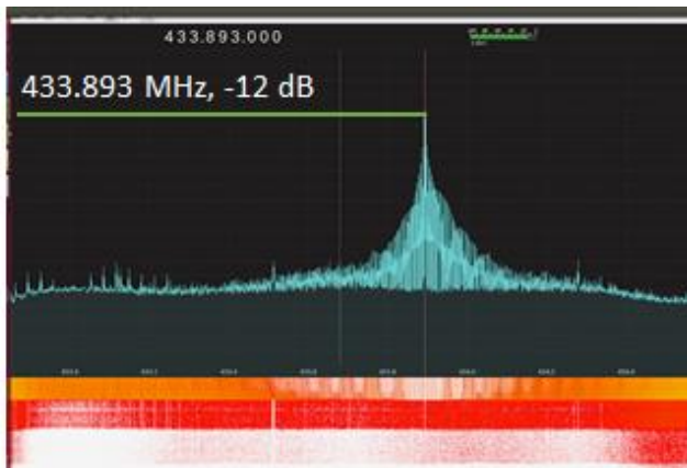
Figure 8: Received Power Spectral Density after OOK modulator is turned on
